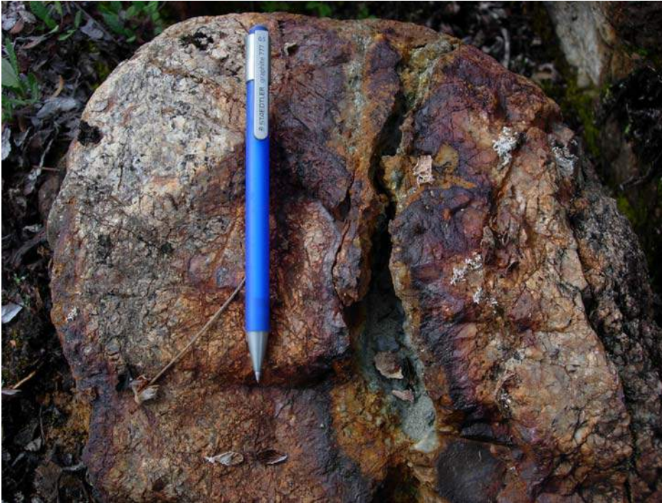
Photo 3: Camp Zone quartz vein with a central portion of auriferous pyrite. UTM 382811-6298677.
