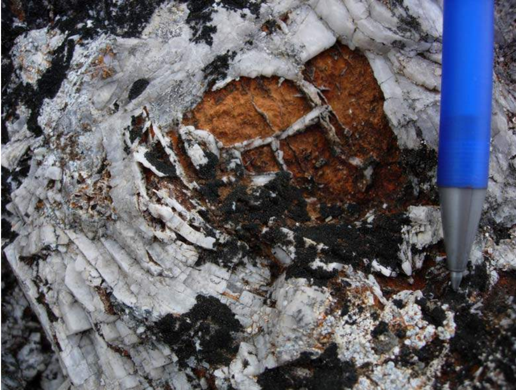
Photo 18: North Cuba Zone. Late coarse barite overgrowing earlier Fe carbonate. UTM 386990-6304434.
