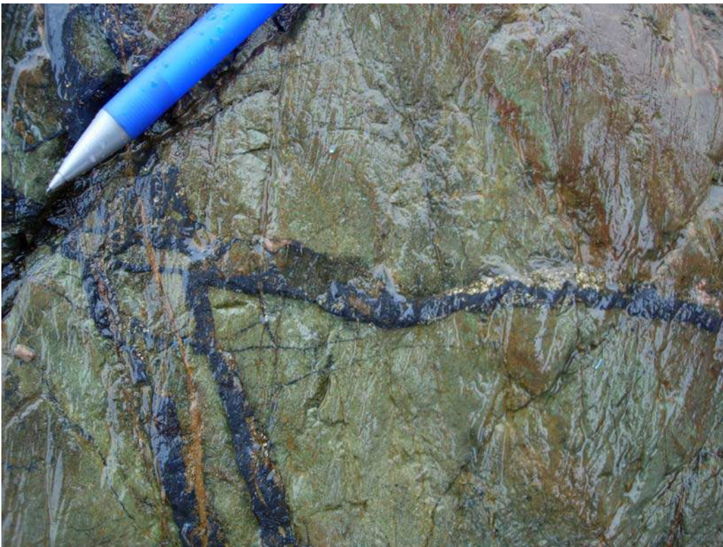
Photo 6: Ken Zone. Epidote-chlorite-altered andesites cut by magnetite-pyrite veins. UTM 3811-6305125.
