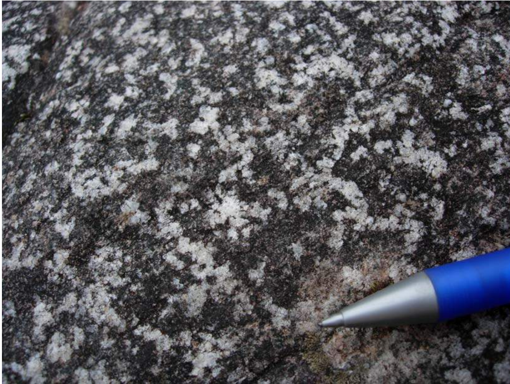
Photo 2: Camp Stock quartz porphyry (Unit QP) with large pale quartz phenocrysts set in a pale to dark grey quartz-feldspathic groundmass. UTM 382749-6298793.
